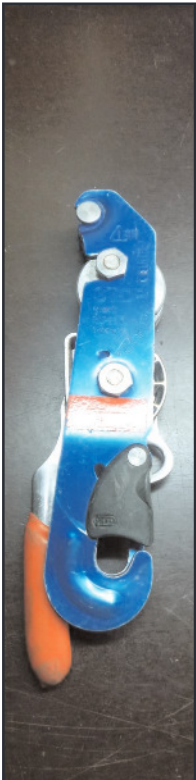
Photo 1: Petzl Stop in closed position. Photo: Chris Curtis.
