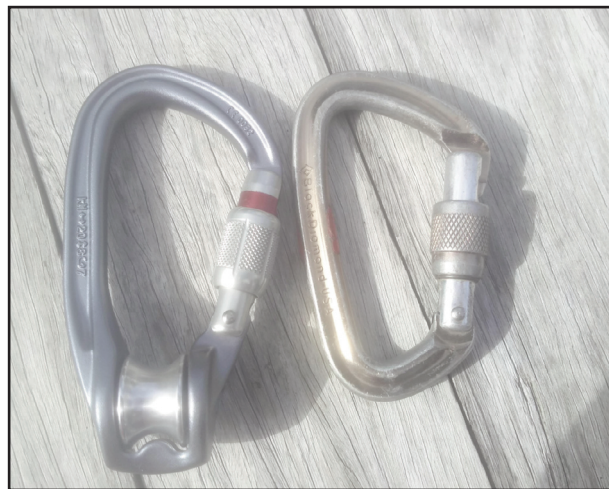
Photo 4: A Petzl Rollclip "Z" Screw-Lock pulley compared to a standard carabiner. Photo: Chris Curtis.
