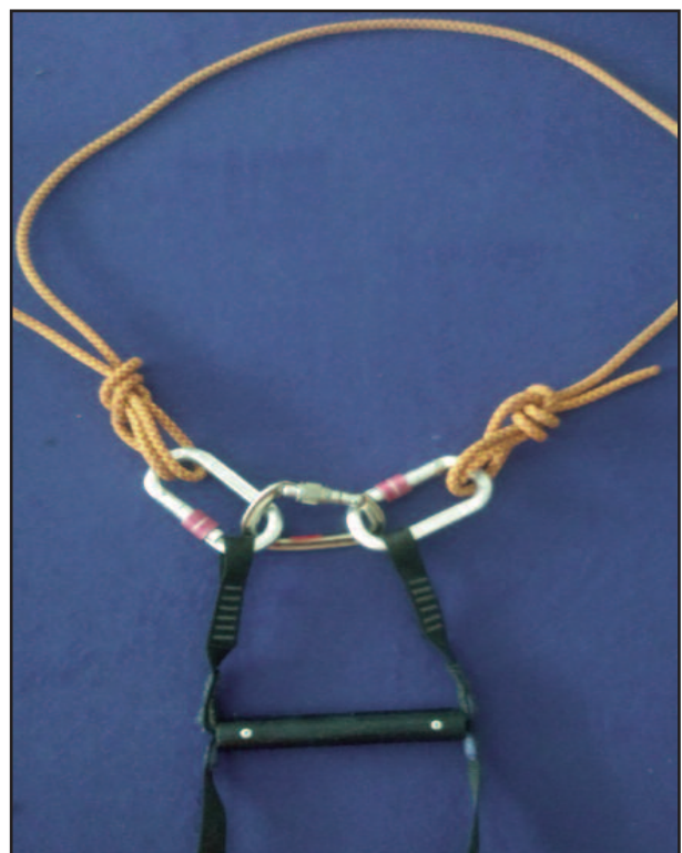
Photo 8: Rigging around large anchors. Photo: Chris Curtis.
