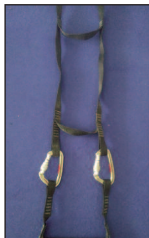
Photo 6: Joining two tape sling ladders. Photo: Chris Curtis.
